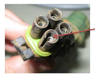
In the above instance the connector pin (PIN B – Main power pin) was corroded. Without careful inspection this fault was missed. The unit reported sensors failing and an un-reliable display module. The fault inspection determined that the electrical pin had a large voltage drop across it causing the LMS system to lose power.
