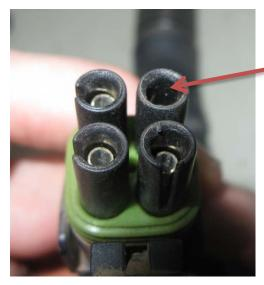
In the above example a connector pin has been backed out of the connector. This causes an intermittent electrical connection and loss of display power. The IO Module was returned for warranty however no faults other than the connector were found.
