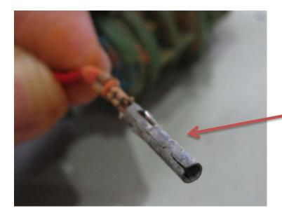
The above instance shows a crimp terminal that is tarnished. This causes a voltage drop across the connector, or total loss of LMS power.
