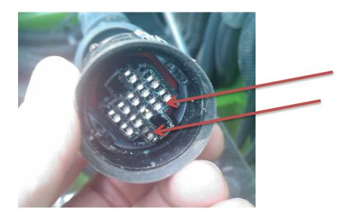
The above image shows blue copper oxide around the connectors as well as one connector pin badly tarnished. In this instance the connector must be changed, cleaning will not suffice.
