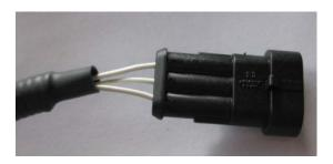
• The control panel harness is a 4 pin female connector with male terminals. The harness is still fitted with orange, purple and yellow wires. It mates with a 4 pin male connector on the system harness.
