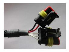
The camera power connector is fitted with a 2 pin connector.
