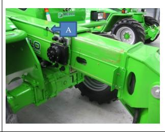
3 Use magnets (not provided) or masking tape to hold the boom clips in place whilst the silicon cures.
