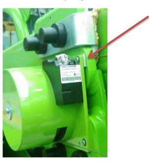
Route the network data cable and secure with a P-clip. Use a M5 x 12mm socket head cap screw, M5 washer and P-Clip as demonstrated in the image (F) below:
