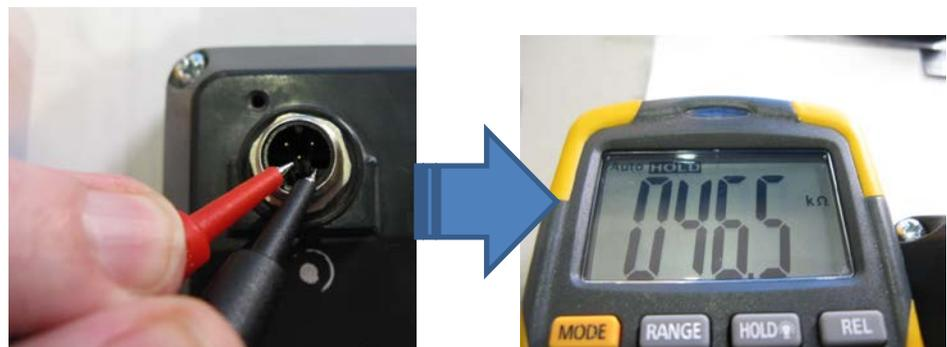
Finally check the integrity of the network data cable and its termination resistors. Use a multimeter with long tipped probes, or use some lengths of wire, paper-clips, etc. and probe the centre pin and the LOWER LEFT HAND PIN of the connector leading into the display (located on the cab wall). Place the positive lead in the centre and the negative lead on the lower left hand pin. You should measure about 60.5 OHMS of resistance.
